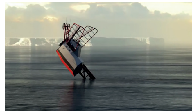
▲ When flooded at the bow, it will flip to a vertical position
